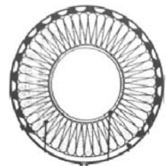
Pipe with thermal insulation and TEMAFOIL™ in between
